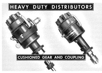
Heavy-duty distributors, as well as some passenger car types, have taken on a new appearance with many added improvements. Torsional vibration, aggravated by higher compression engines, made shock-absorbing distributor drives a necessity. Both gear and coupling drives
